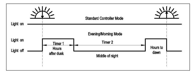
The MP-3735 recognizes days and night based on the solar array voltage. NLF will start when the PV(Voltage) < 10V for a period of time.
